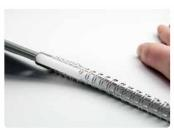
Slide the device all the way along the wire seam.
