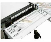
Automatic binding table clamps the media and holds the blocks in place during binding. It then ejects the book or calendar blocks automatically up to 60% more productive than a standard binding table.
